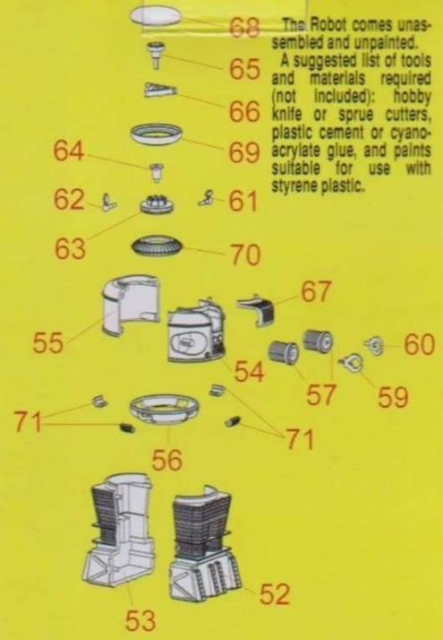
Cement Robot Bottom Halves (#52 and #53) together, and then set them aside. Cement Small Clear Parts (#71) into Lower Ring of Body (#56) cement Enunciator (#67) into Body Front Half (#54) cement Body Halves (#54 and #55) together, then cement Bottom Ring (#56) in place.
